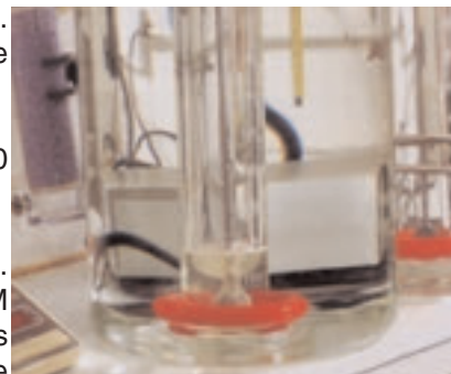
Example of Non-Foaming Oil.
